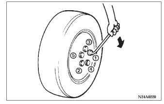
11. Lower the vehicle slowly and then tighten the nuts in the sequence shown in the illustration until each nut has been tightened to the specified torque.
